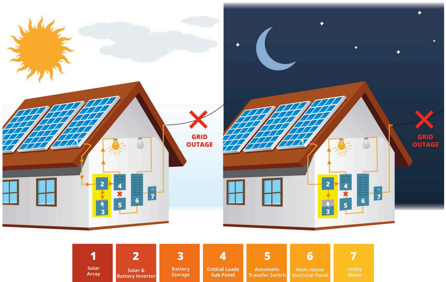
A diagram showing how a battery and solar system operates when there is a grid outage both during the day and at night.
